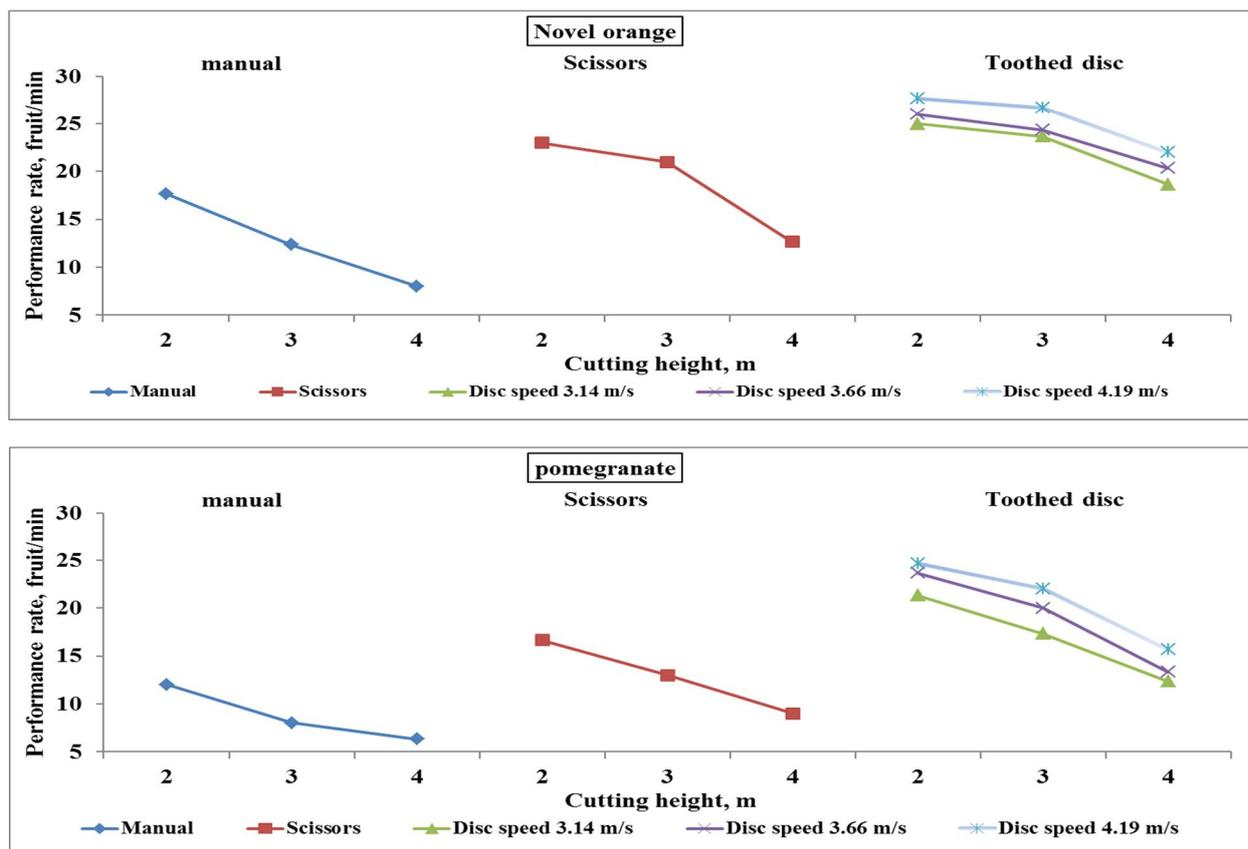
**Fig. 6:** Effect of some operating parameters on machine performance rate for harvesting navel orange and pomegranate fruits
