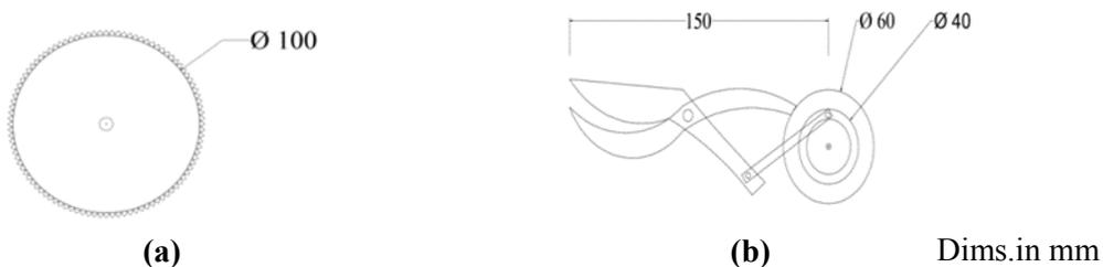
**Fig. 3:** Schematic views of the different cutter head types: (a) toothed disc (b) scissor
