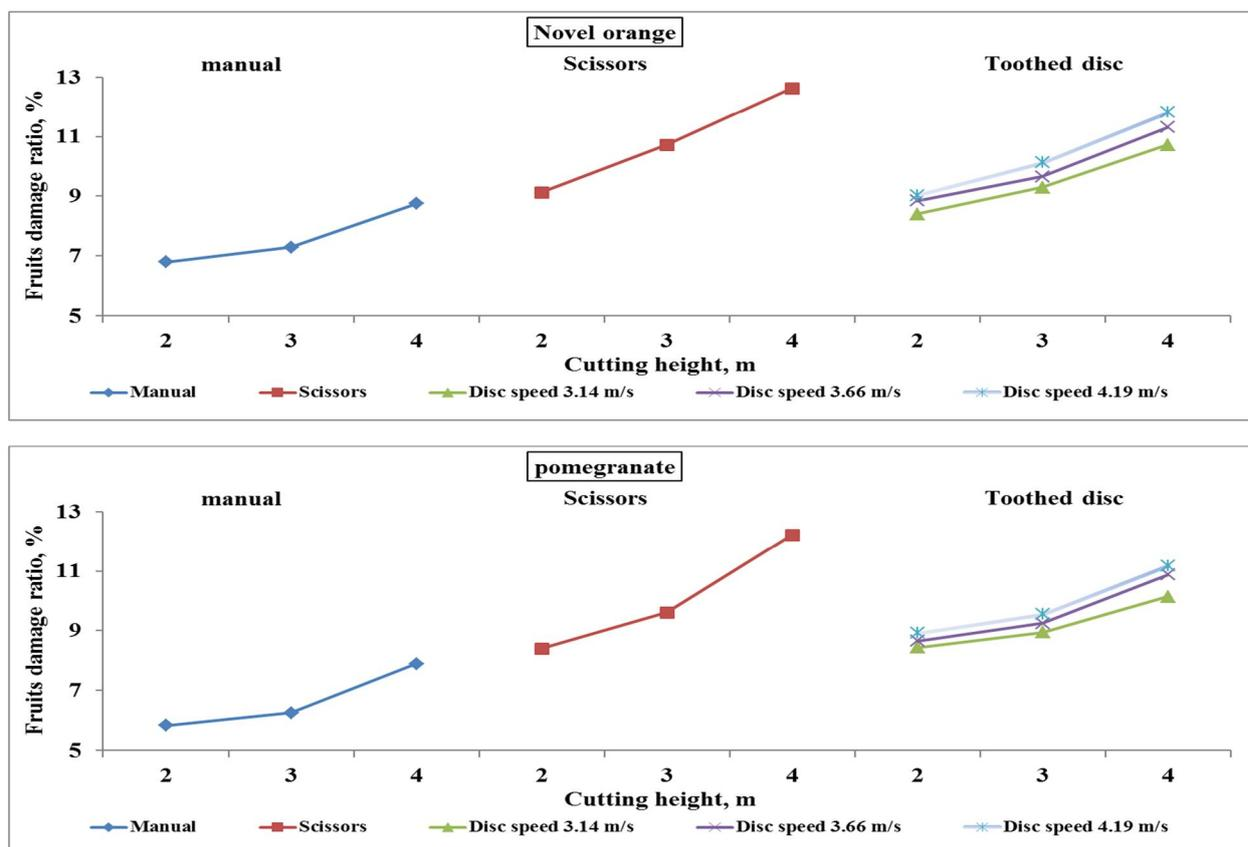
Fig. 7: Effect of some operating parameters on fruits damage ratio for harvesting navel orange and pomegranate fruits
