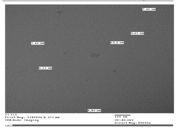
**Image 2:** TEM of selenium Nano-particles size, demonstrate ranged diameter in nanometer between (6.53 – 10.6) nm.
