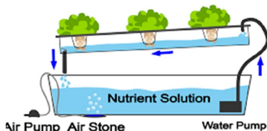
Fig. 9: Nutrient film technique (NFT)
