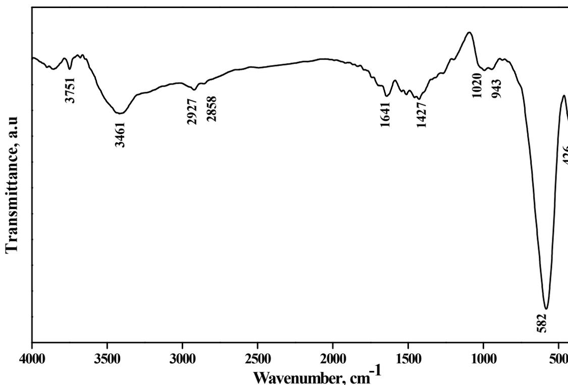
Fig. 2: FTIR spectrum of the prepared  $\text{CoFe}_2\text{O}_4$  nanoparticles.
