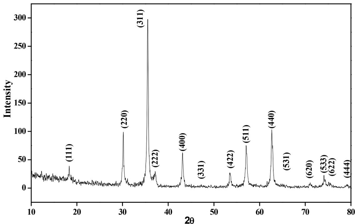
Fig. 1: X-ray diffraction (XRD) pattern of the prepared CoFe<sub>2</sub>O<sub>4</sub> nanoparticles.
