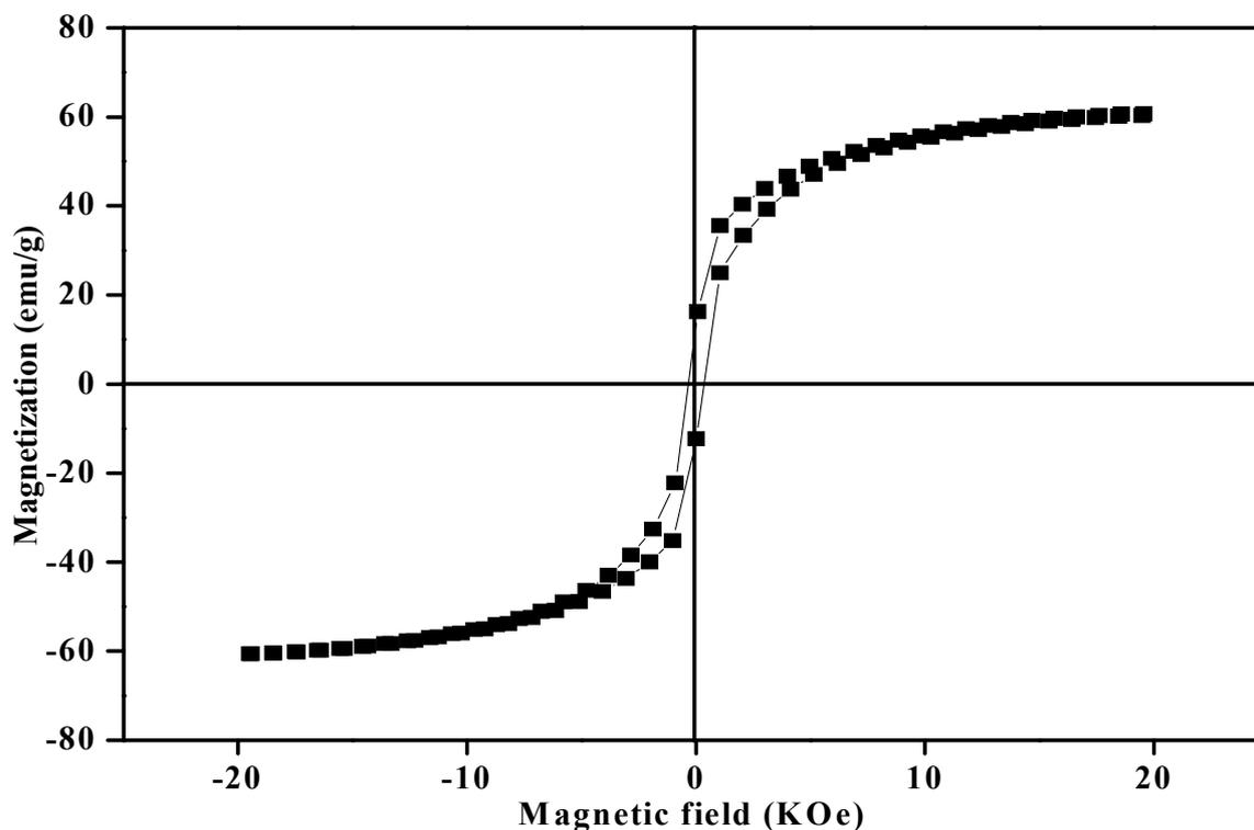
Fig. 3: Hysteresis loop of the prepared  $\text{CoFe}_2\text{O}_4$  nanoparticles.
