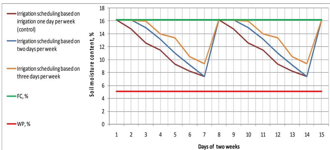
**Fig. 3:** Effect of irrigation scheduling under rotational irrigation system on water stress on citrus trees (Noval orange, Lemon, Sour orange and Grapefruit)
