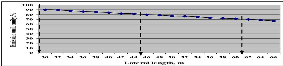
Fig. 3: The relation between emission uniformity and increasing of lateral length (Lateral length 30 m, 46 m, and 62 m appropriate with emission uniformity 90%, 80%, and 70% respectively)
