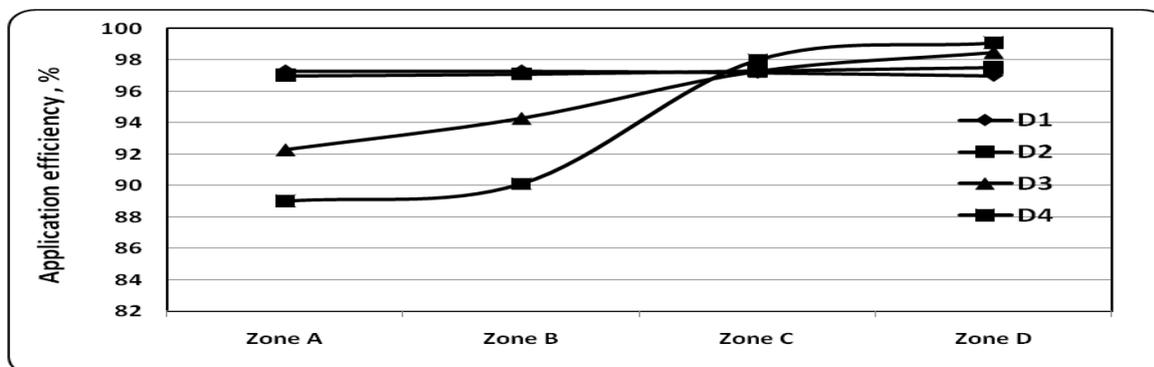
**Fig. 5:** Effect of volumetric distribution ratios of compost on four zones along lateral on application efficiency under 90% emission uniformity.
