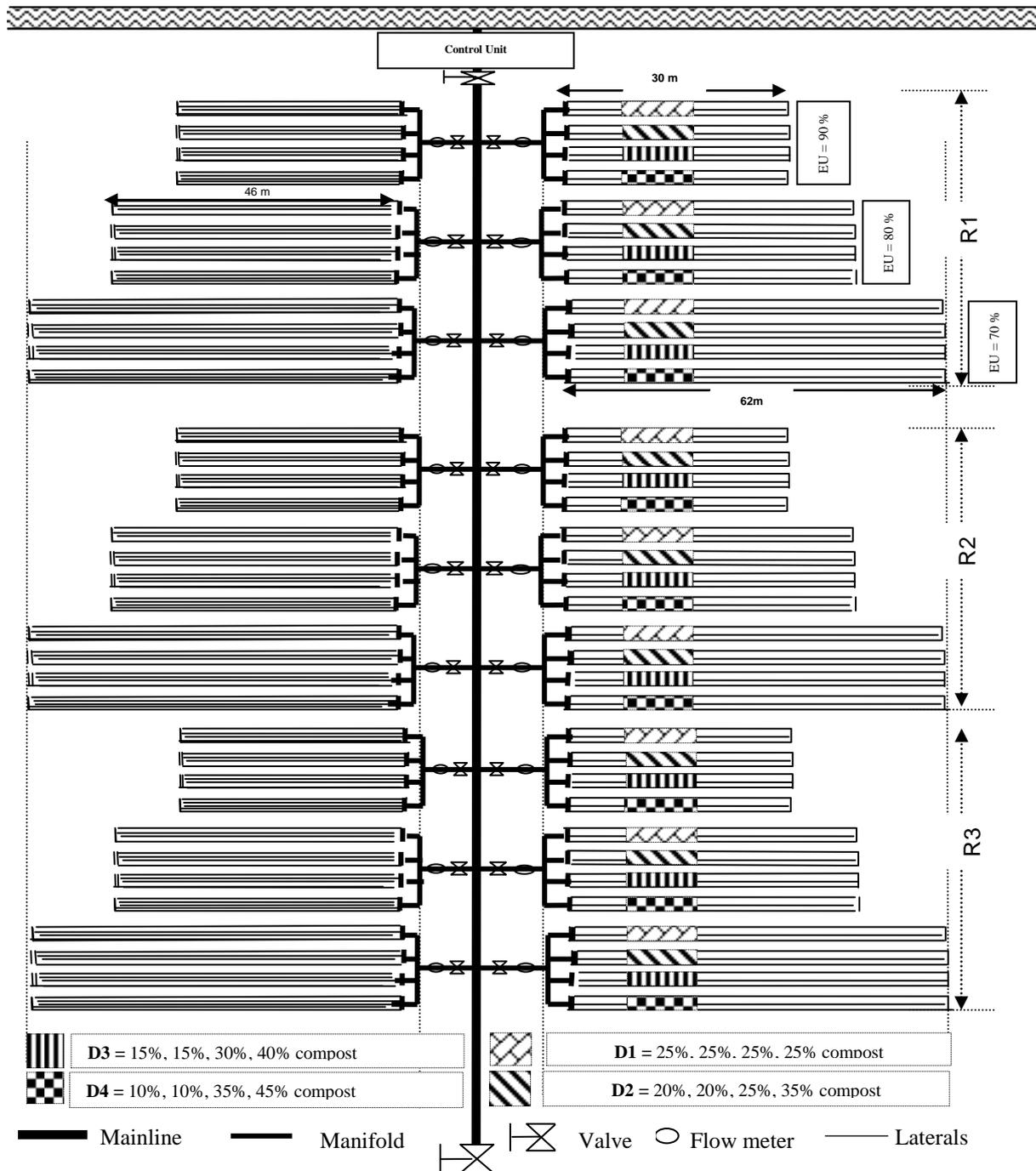
Fig. 4: Schematic diagram for the experiment design layout.
