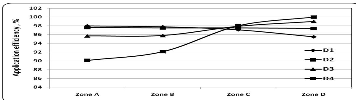
**Fig. 6:** Effect of volumetric distribution ratios of compost on four zones along lateral on application efficiency under 80% emission uniformity.
