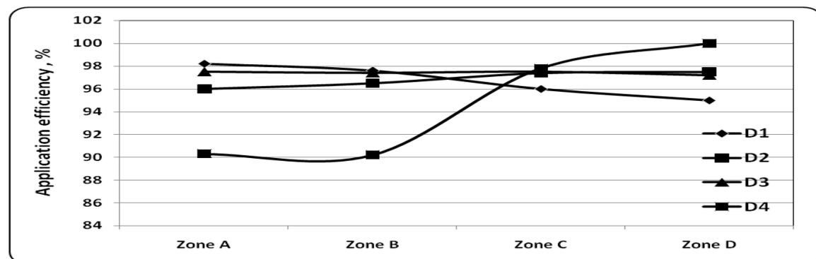
**Fig. 7:** Effect of volumetric distribution ratios of compost on four zones along lateral on application efficiency under 70% emission uniformity.
