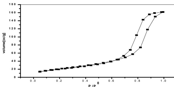
Fig. 5: BET of the adsorbent
