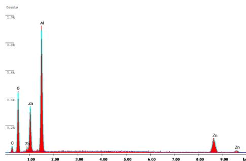
Fig. 3: EDX of the adsorbent
