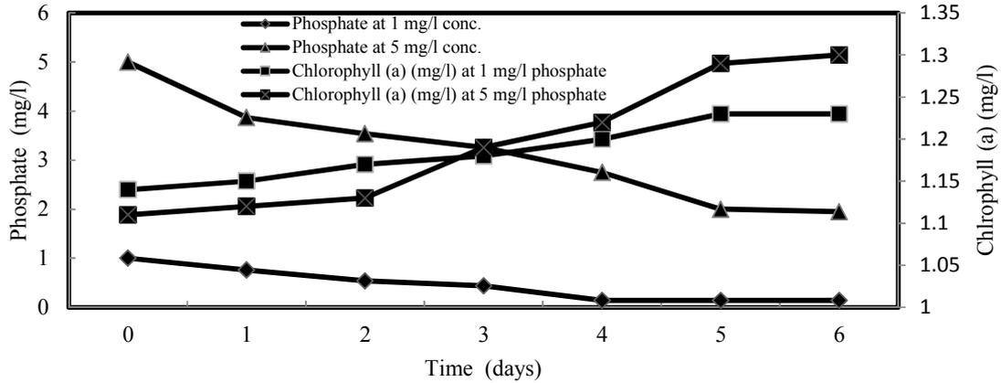
**Fig. 6:** Time course of phosphate removal and development of chlorophyll (a) at concentration ratio (95%). ( $[\text{PO}_4^{3-}] = 1 \text{ mg/l}$  &  $[\text{PO}_4^{3-}] = 5 \text{ mg/l}$ )
