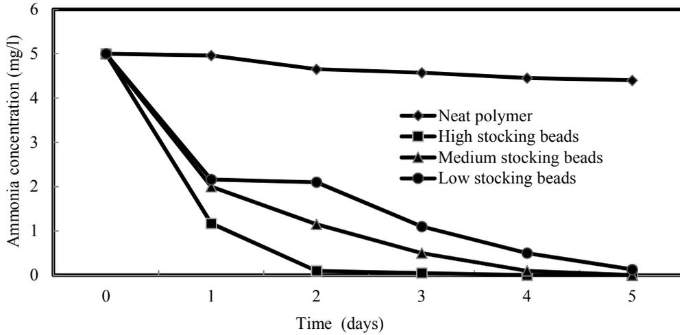
**Fig. 9:** Effect of time on the removal of ammonia, using low, medium and high stocking beads. ( $[\text{NH}_3] = 5$  mg/l)
