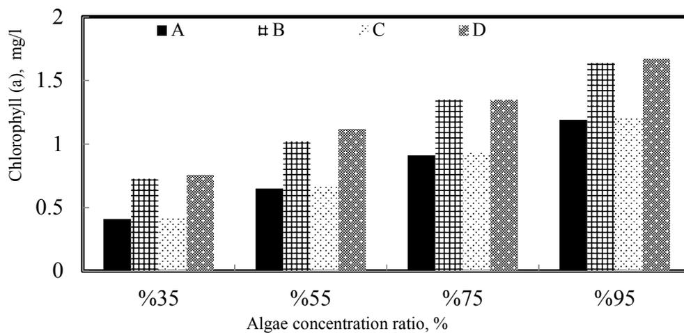
**Fig. 5:** Effect of algal concentration ratio on the developed concentration of chlorophyll (a). ( $[\text{NH}_3] = 1 \text{ mg/l}$  and  $[\text{NH}_3] = 5 \text{ mg/l}$ )
