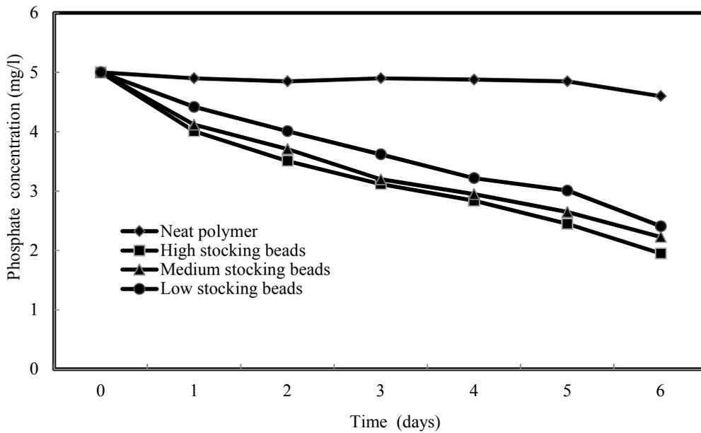
**Fig. 10:** Effect of time on the removal of phosphate, using low, medium and high stocking beads. ( $[\text{PO}_4^{-3}] = 5$  mg/l)
