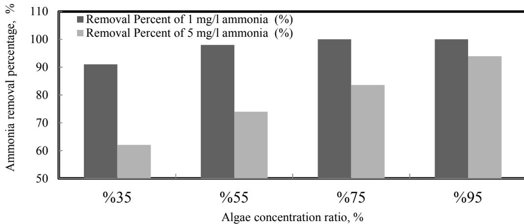
**Fig. 4:** Effect of algal concentration ratio on the removal percent of ammonia. ( $[\text{NH}_3] = 1 \text{ mg/l}$  &  $[\text{NH}_3] = 5 \text{ mg/l}$ ).
