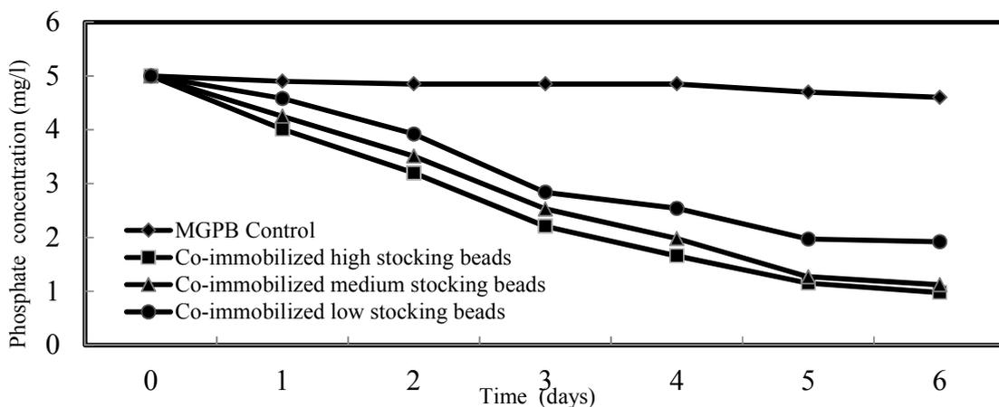
**Fig. 12:** Effect of time on the removal of phosphate, using co-immobilized low, medium and high stocking beads. ( $[\text{PO}_4^{3-}] = 5 \text{ mg/l}$ )
