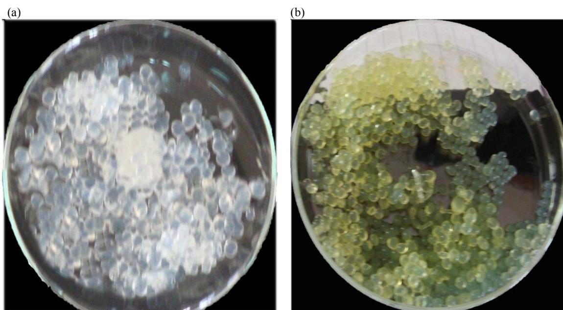
**Fig. 2:** Simple picture by digital camera of neat polymer (a) and immobilized microalga beads (b).
