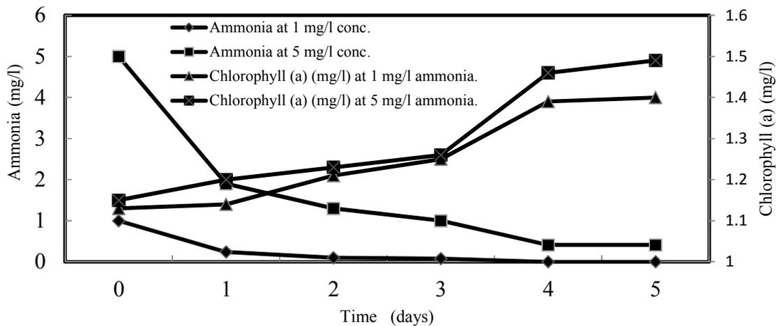
**Fig. 3:** Time course of ammonia removal and development of chlorophyll (a) at concentration ratio (95%). ([NH<sub>3</sub>] = 1 mg/l & [NH<sub>3</sub>] = 5 mg/l)
