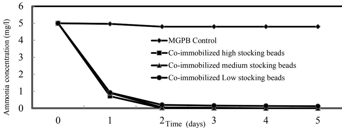
**Fig. 11:** Effect of time on the removal of ammonia, using co-immobilized low, medium and high stocking beads. ( $[\text{NH}_3] = 5 \text{ mg/l}$ )
