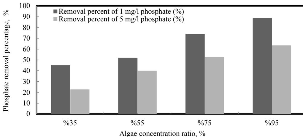
**Fig. 7:** Effect of algal concentration ratio on the removal percent of phosphate. ( $[\text{PO}_4^{3-}] = 1 \text{ mg/l}$  &  $[\text{PO}_4^{3-}] = 5 \text{ mg/l}$ )
