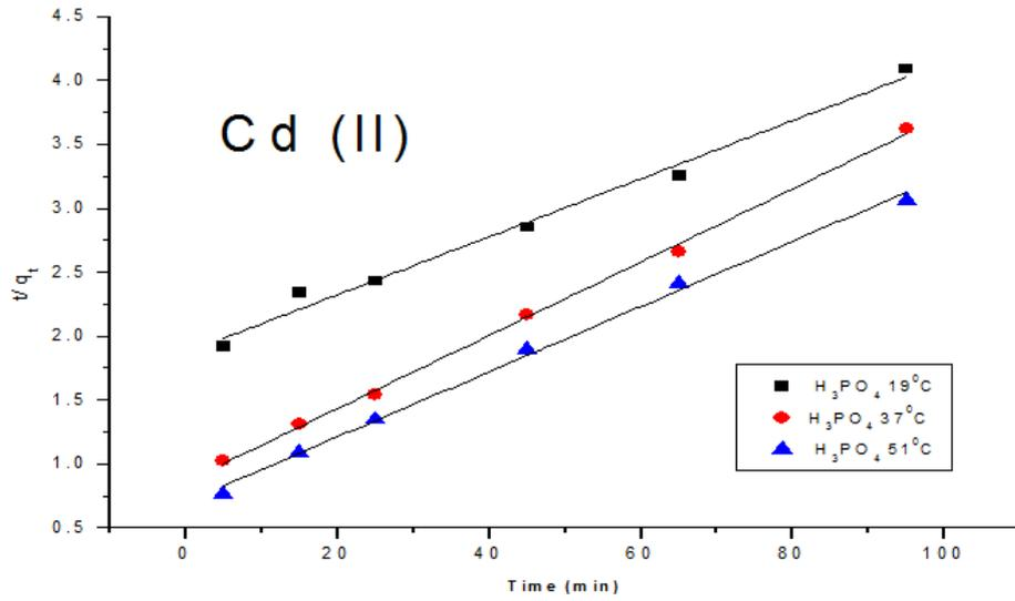
**Fig. 7a:** Pseudo second order plot for the Cd (II) adsorption (8mm ol/ L) by resinx K-8 in the presence of H<sub>3</sub>PO<sub>4</sub> 0.1M
