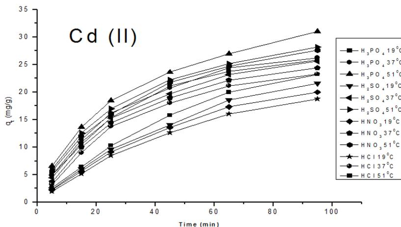
**Fig. 9:** Effect of different temperatures on the adsorption of Cd (II) 8mm ol/L in the presence of some inorganic acids.
