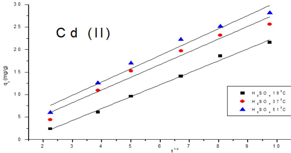
**Fig. 8b:** Weber plot for the Cd (II) adsorption (8mm ol/ L) by resinx K-8 in the presence of  $H_2 PO_4$  0.1M at different tem pretures
