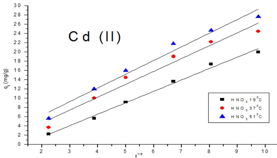
**Fig. 8c:** Weber plot for the Cd (II) adsorption (8mm ol/ L) by resinx K-8 in the presence of  $HNO_3$  0.1M at different tem pretures
