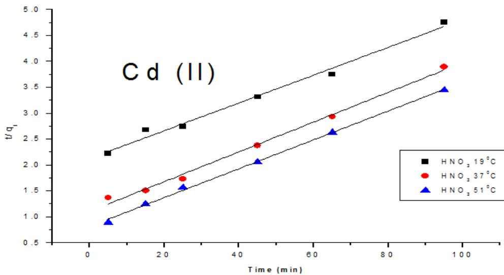
**Fig. 7c:** Pseudo second order plot for the Cd (II) adsorption (8mm ol/ L) by resinx K-8 in the presence of H<sub>2</sub>SO<sub>4</sub> 0.1M
