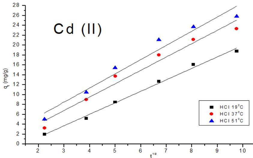
**Fig. 8d:** Weber plot for the Cd (II) adsorption (8mm ol/ L) by resinx K-8 in the presence of HCl 0.1M at different tem pretures
