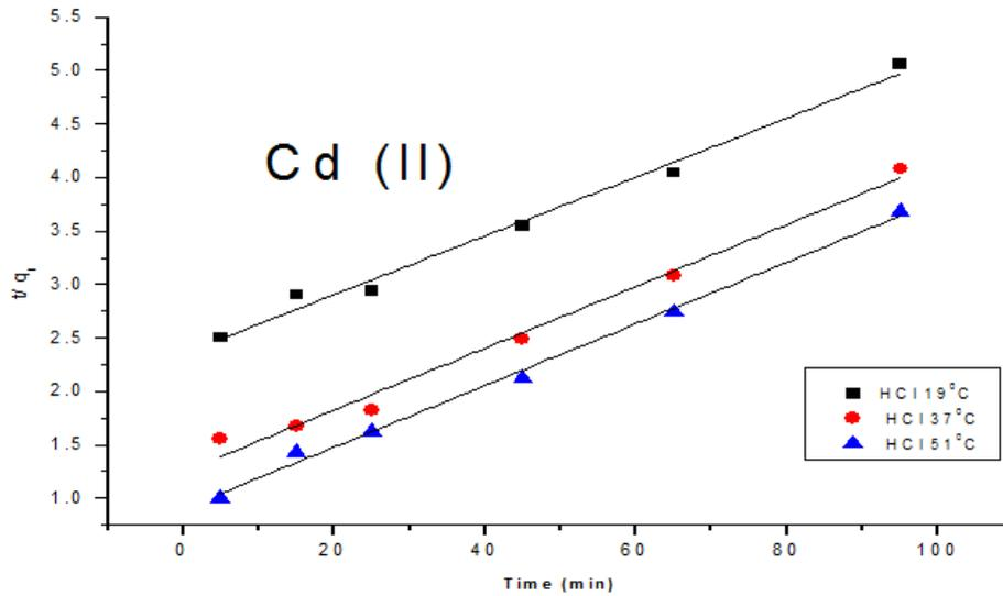
**Fig. 7c:** Pseudo second order plot for the Cd (II) adsorption (8mm ol/ L) by resinx K-8 in the presence of HCl 0.1M
