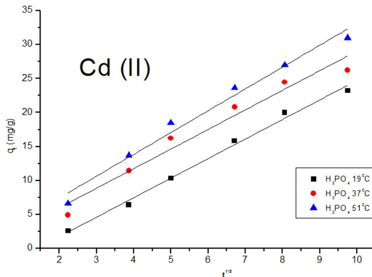
**Fig. 8a:** Weber plot for the Cd (II) adsorption (8mm ol/ L) by resinx K-8 in the presence of H<sub>3</sub> PO<sub>4</sub> 0.1M
