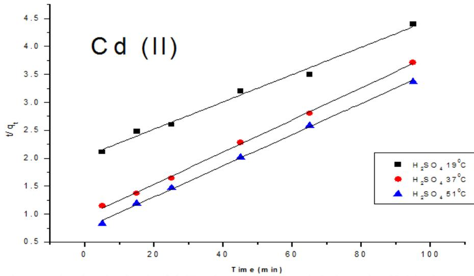
**Fig. 7b:** Pseudo second order plot for the Cd (II) adsorption (8mm ol/ L) by resinx K-8 in the presence of H<sub>2</sub>SO<sub>4</sub> 0.1M
