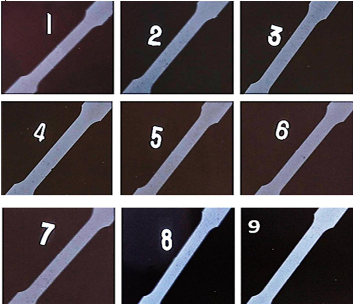
**Fig: 3.** Photo of porosity formation and their distribution in tensile
