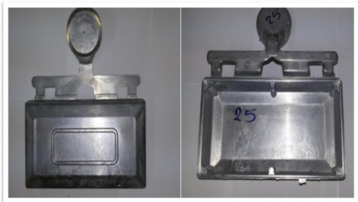
**Fig. 1:** Final sample of material of ADC12 after casting
