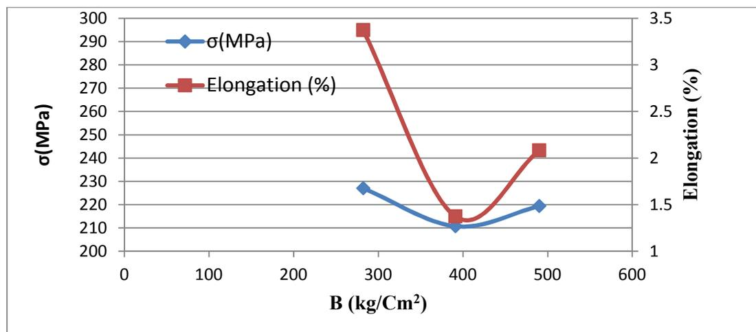
**Fig. 6:** Tensile test results at the different Multiplied Pressure Under (650 (°C) and 3 (m/s))
