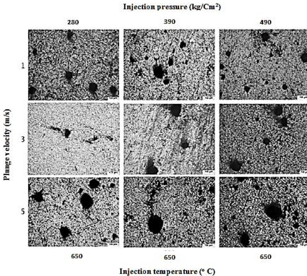
**Fig. 2** Effect of holding furnace temperatures (injection temperature) (650°C) with different multiplied pressure (280,390,490(kg /cm<sup>2</sup>)) and different plunger velocity of 2nd stage (1, 3, 5 (m/s)) on the porosity formation.
