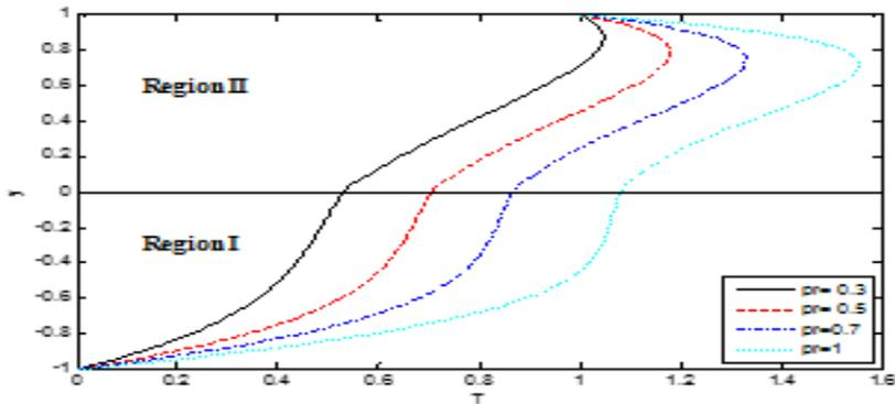
**Fig. 9:** Effect of Prndtle number on the fluid temperature.
