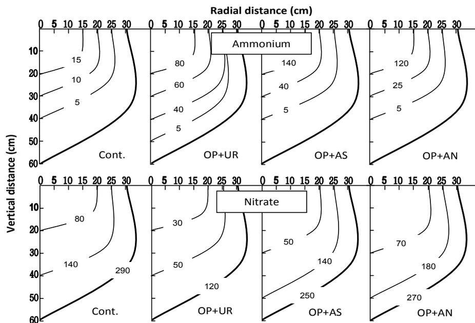
**Fig. 3:** Spatial distributions of ammonium and nitrate ( $\text{mg kg soil}^{-1}$ ) in the root zone as affected by fertigation of OP and different forms of nitrogen at the end of last fertigation cycle. The heavy peripheral lines are the position of the wetting fronts.
