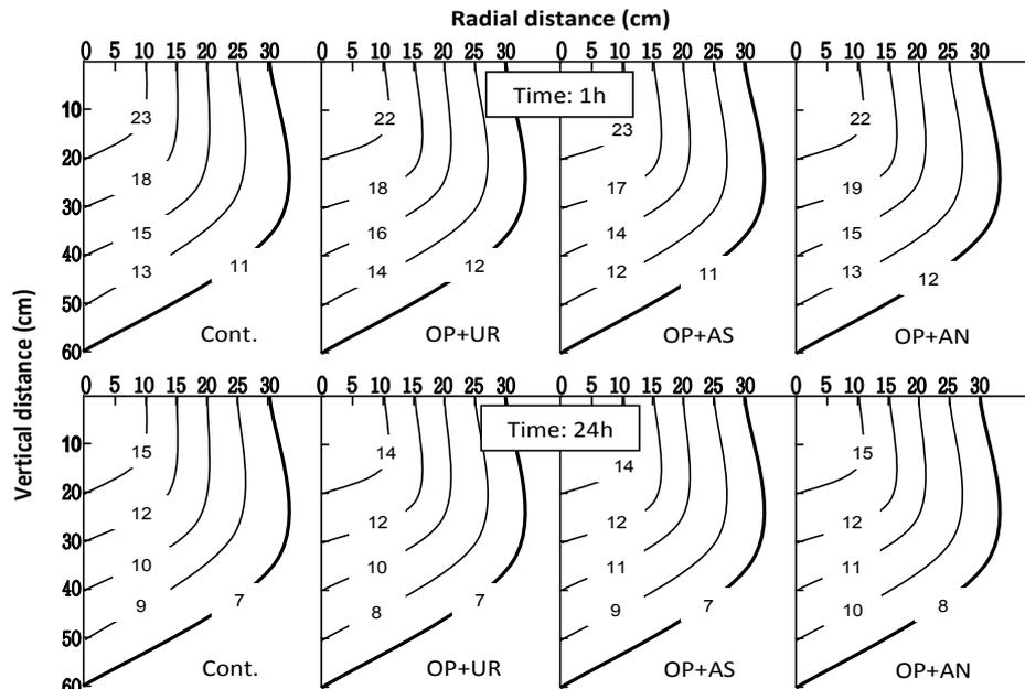
**Fig. 1:** Soil moisture distribution (%) in the root zone at the end (Time: 1h) and before the next (Time: 48h) of third irrigation cycle. The heavy peripheral lines are the position of the wetting fronts.
