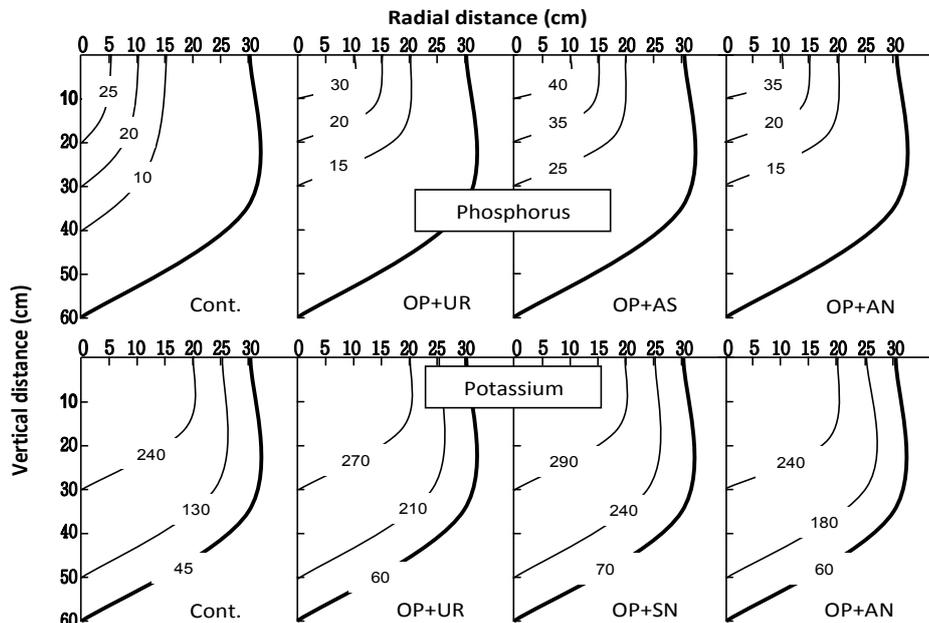
**Fig. 4:** Spatial distributions of phosphorus and potassium ( $\text{mg kg}^{-1}$  soil) in the root zone as affected by fertigation of OP and different forms of nitrogen at the end of last fertigation cycle. The heavy peripheral lines are the position of the wetting fronts.
