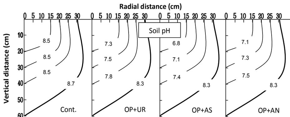
**Fig. 2:** Temporally changes in soil reaction (pH) as affected by fertigation of OP and different forms of nitrogen in the root zone at the end of last fertigation cycle. The heavy peripheral lines are the position of the wetting fronts.
