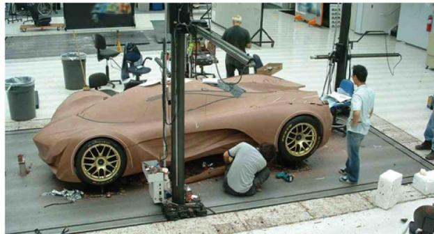
Fig.15: Illustrates the first sample models (prototype) building
