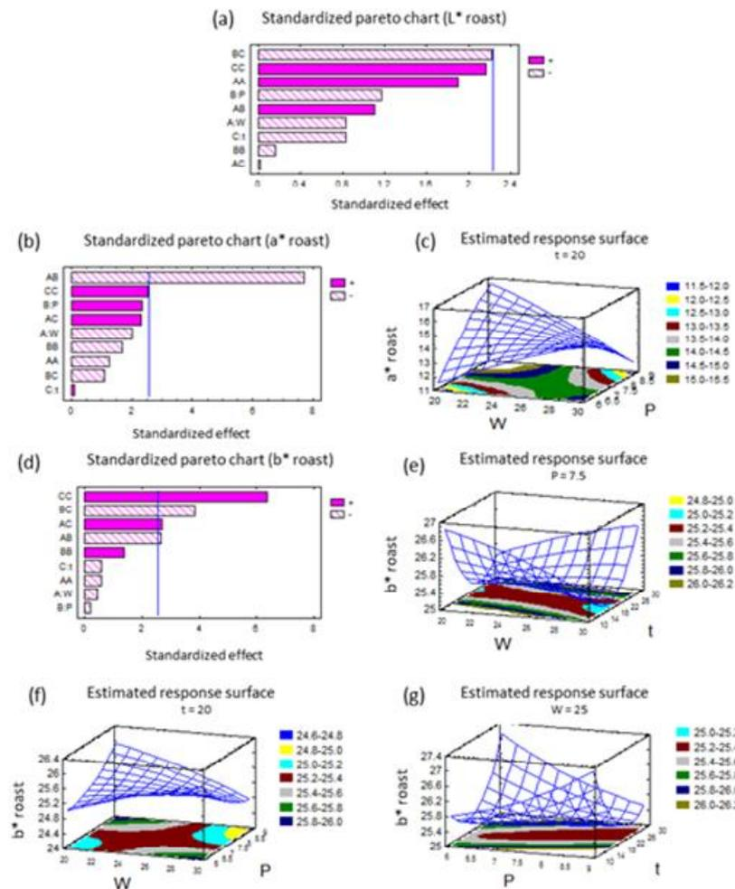
**Fig. 4:** (a, b, d) Standardized Pareto charts and (c, e, f, g) Response surface plots of operating parameters (A = W, B = P and C = t) on the color (L\*, a\* and b\*) of Maize C after expansion (exp) and roasting (roast).
