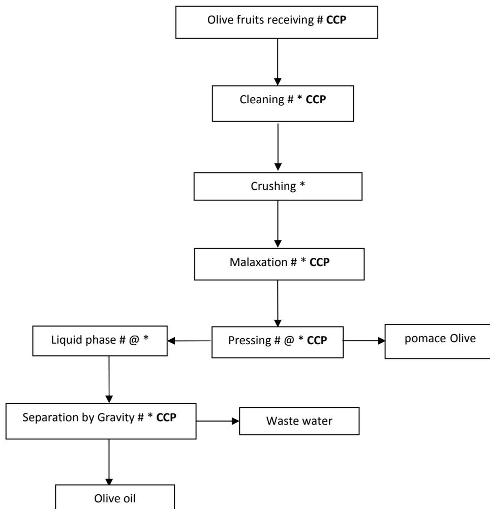
**Fig. 1.** Flow diagram of the extraction olive oil by hydraulic press method.
