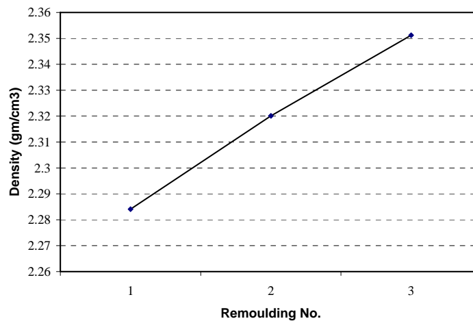
Fig. 3: Effect of remoulding process on mix density for mix 3D
